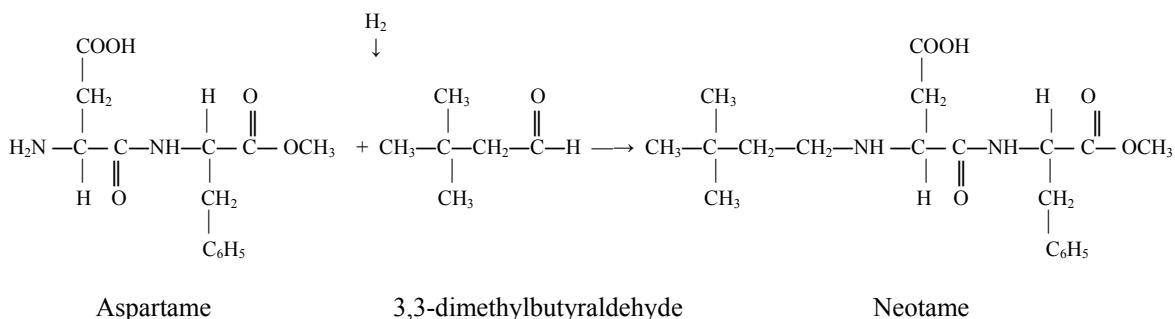
The isolation and purification of neotame is carried out by the distillation of a portion of the methanol followed by the addition of water (approximately 2.5 litres per mole aspartame). The mixture is cooled for a number of hours and neotame is then isolated by an appropriate solid/liquid separation method such as centrifugation. Additional water is used to wash the product, which is then dried in appropriate equipment (e.g. a vacuum drier).
